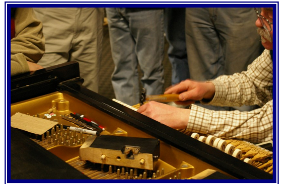
Below: Tony demonstrates the ball peen hammer voicing technique.
